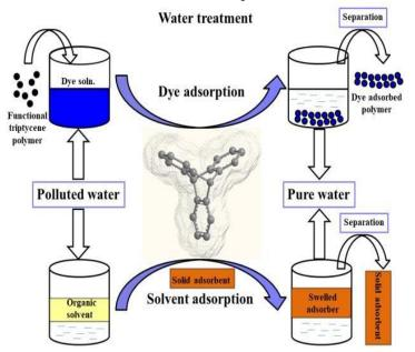
Triptycene-based functional polymers for the removal of micropollutants (organic dyes and solvents).
